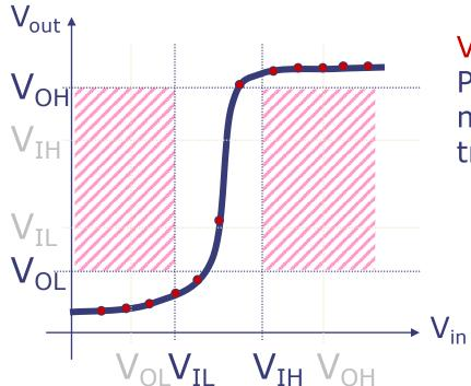
Voltage Transfer Characteristic (VTC): Plot of  $V_{out}$  vs.  $V_{in}$  where each measurement is taken after any transients have died out
