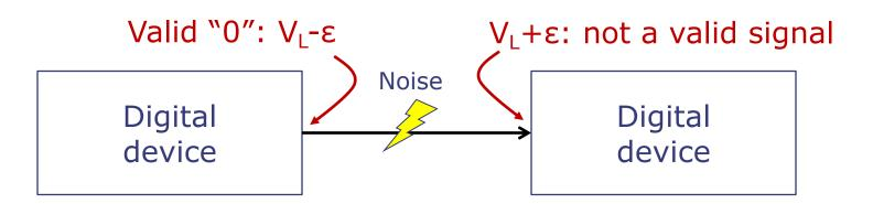
Upstream device transmits a signal at  $V_L$ - $\epsilon$ , a valid "0". Noise on the wire causes the downstream device to receive  $V_L$ + $\epsilon$ , which is undefined.
