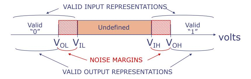
A digital device accepts marginal inputs and provides unquestionable outputs (to leave room for noise)
